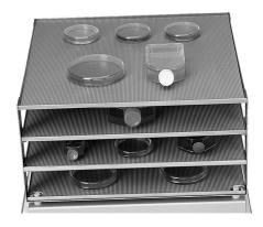
Platform Frames to increase the capacity of the Shaking Apparatus made of stainless steel with 4 levels
