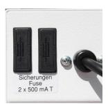
The two fuses of the Shaking Apparatus are situated in a drawer at the back of the unit. In order to check or to exchange these fuses, press the fixing clips on both sides of the drawer and pull.
