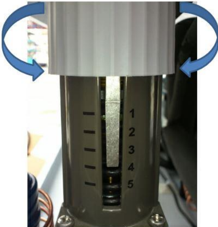
Fig. 3 Turning the dial in direction 1 on the scale increases the amount of cooling water and turning it in direction 5 on the scale reduces the amount of cooling water.
