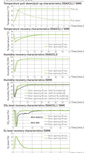
\* MCO-50AlC(L) Ambient temperature: 23°C, setting: 37°C,  $C0_2$ : 5 %, no load \* MCO-50M Ambient temperature: 23°C, setting: 37°C,  $C0_2$ : 5 %,  $0_2$ : 5 %, no load
