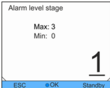
Fig. 47: Specifying level alarm level
