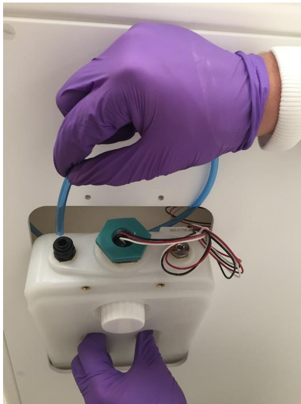
Figure 26: Water Tank top tube removal
