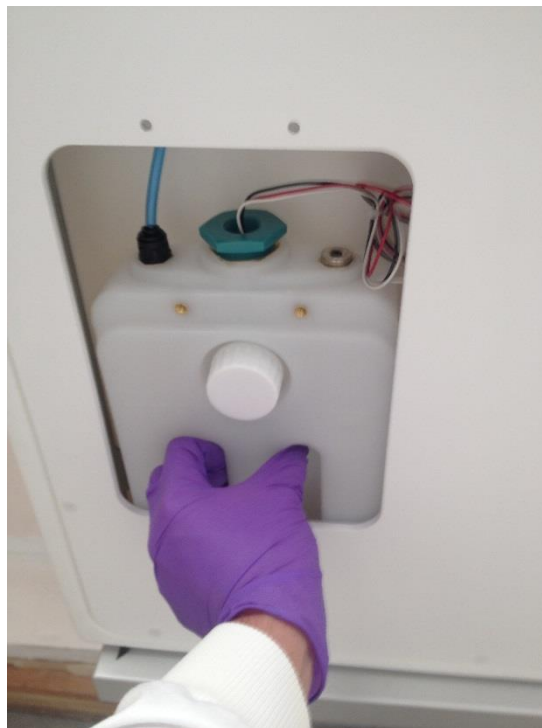
Figure 24: Water Tank lowered for removal
