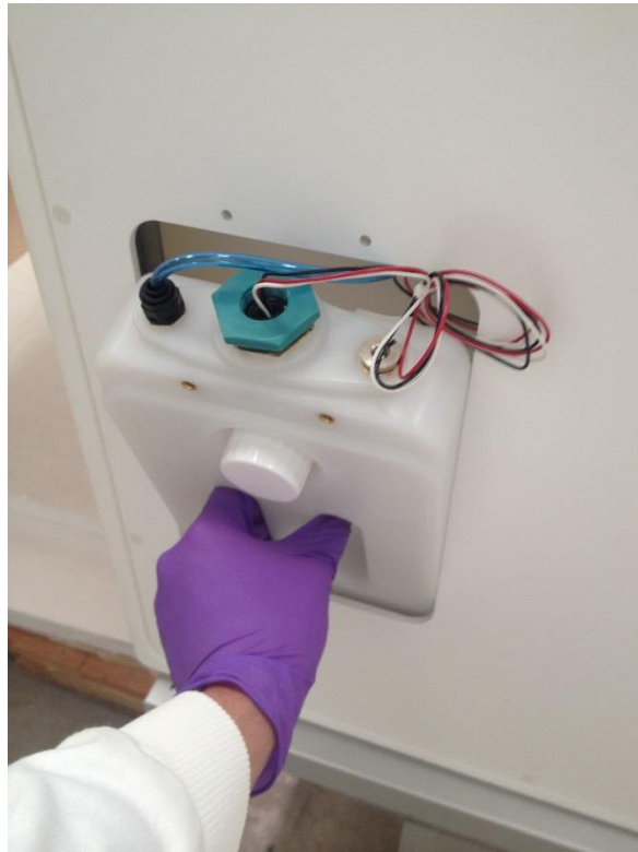
Figure 25: Water Tank tilted forward partially removed
