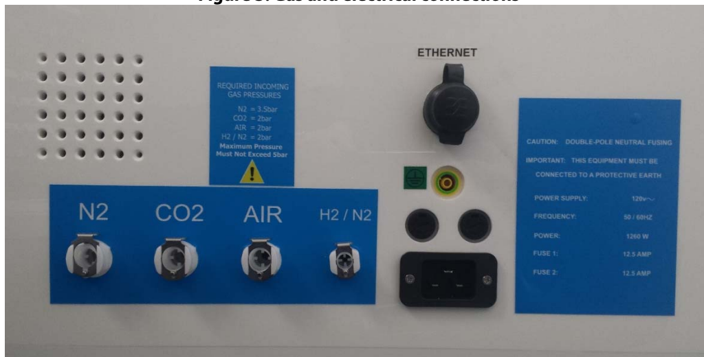
Figure 3: Gas and electrical connections
