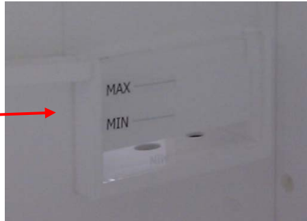
Figure 38: Water tank internal level indicators
