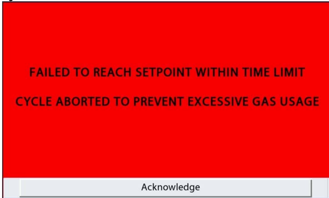
Figure 42: Failure to reach Set Point Alarm
