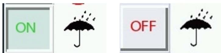
The % relative humidity can be set by entering a % value into the (% RH) Set Point box from the “**Atmosphere Control Screen**”. The % relative humidity can only be set when the humidity system is on and the humidity button indicates a green **ON**.
