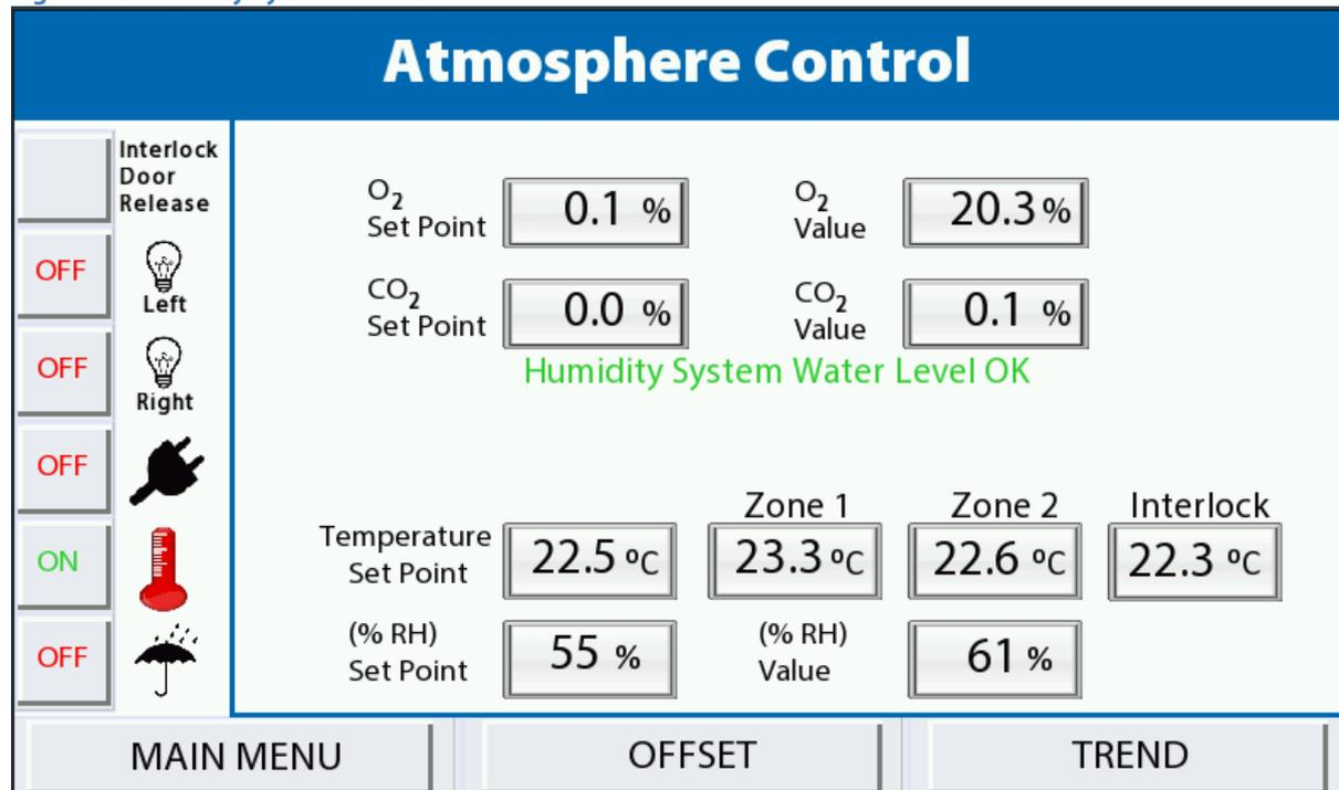
If the humidifier water level is too low, an alarm will sound and an alarm message will be displayed on the control screen as shown in Figure 29.
