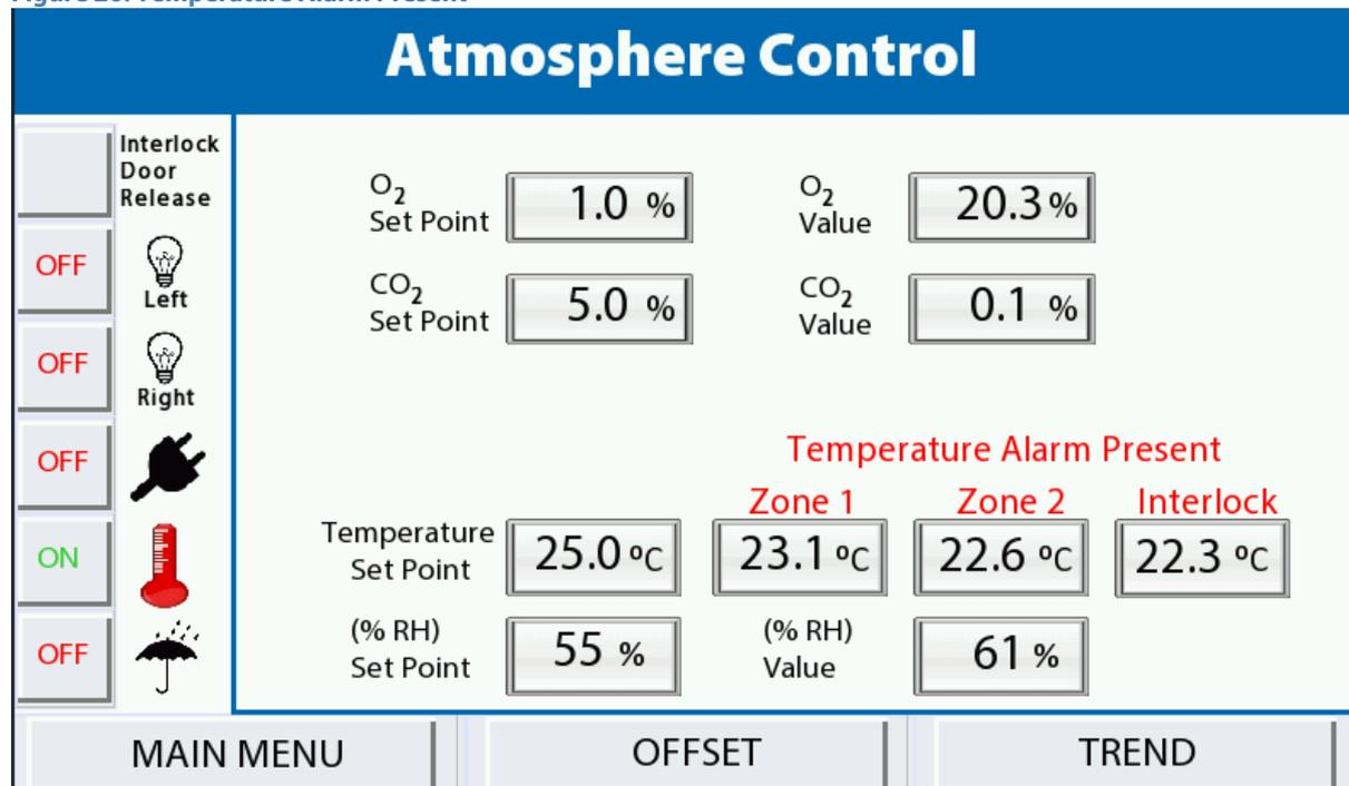
The “**Temperature Alarm Present**” message is displayed on the main Atmosphere Control screen as shown in Figure 26.
