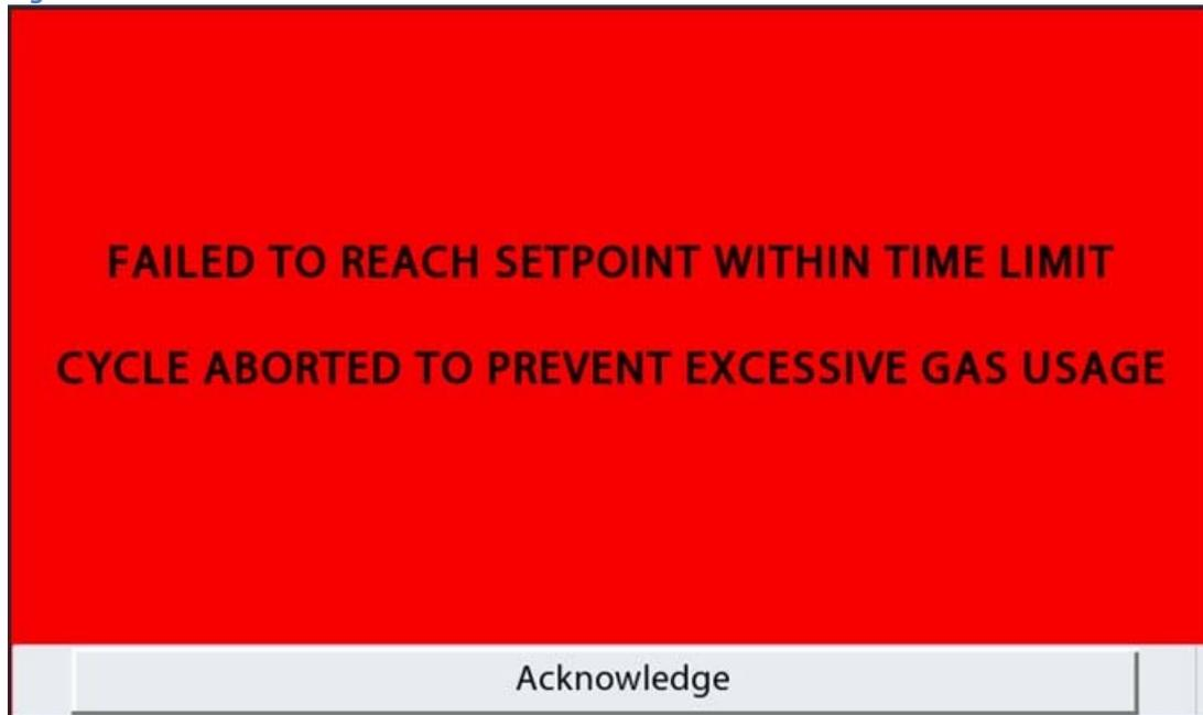
This alarm occurs when the internal control time limit to reach Set point has been exceeded and the cycle is aborted. This function prevents excessive gas usage. It is recommended to adjust the set point and re-start the cycle. If this alarm occurs repeatedly see trouble shooting in Section 6.6.
