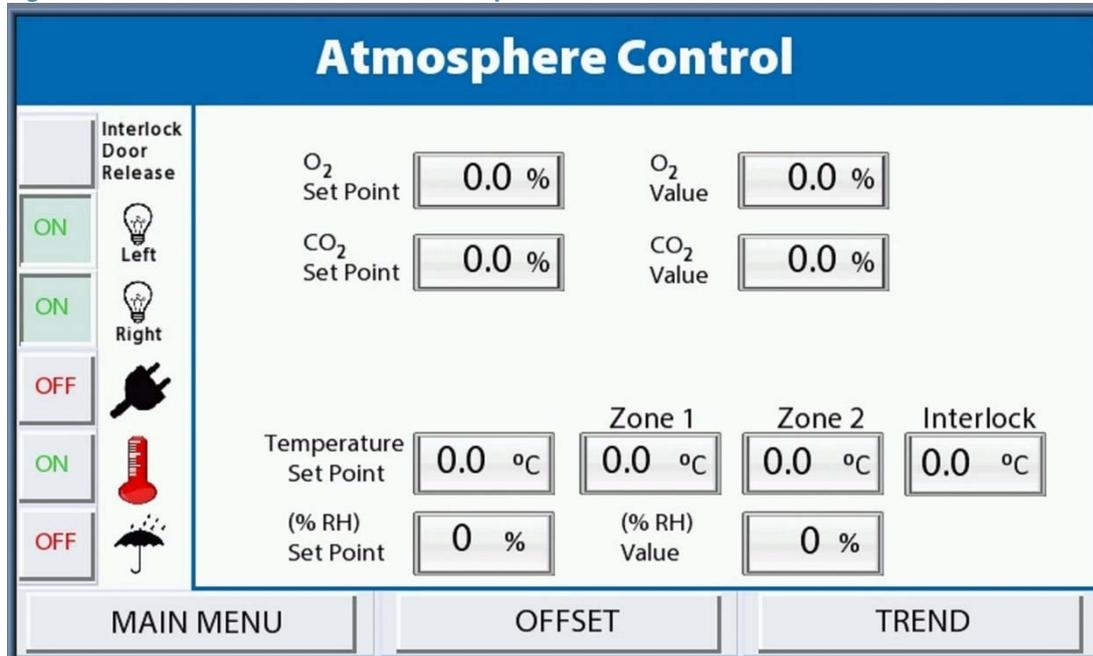
The O<sub>2</sub> Set point and CO<sub>2</sub> Set point can be set using the Atmosphere Control screen as shown above.
