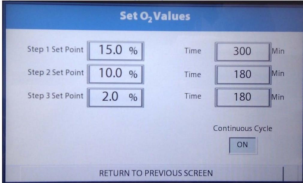
The Continuous Cycle will operate until the cycle is aborted by the user. The Cycle is aborted by pressing the **RETURN TO PREVIOUS SCREEN** button.
