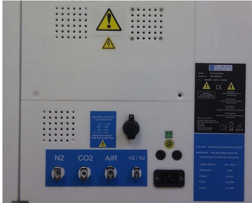
Figure 4 lists the gasses required for operation of the workstation;
