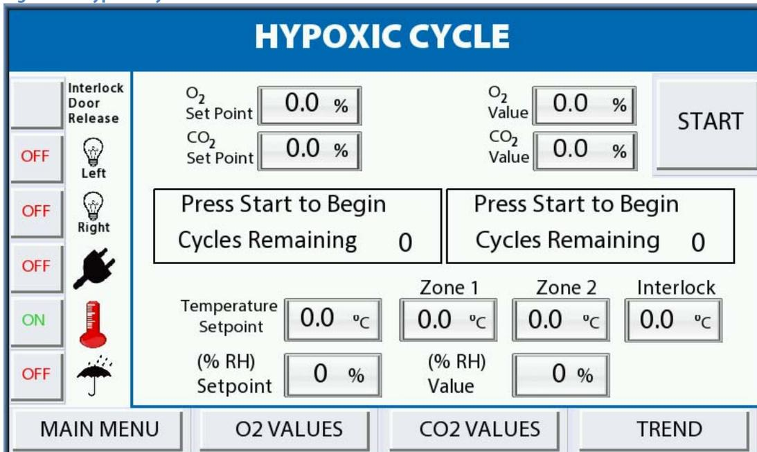
Press the **O<sub>2</sub> VALUES** button to enter O<sub>2</sub> set up screen and the **CO<sub>2</sub> VALUES** button to enter the CO<sub>2</sub> screen. The Cycles will be shown on the main **HYPOXIC CYCLE** screen shown in Figure 38.
