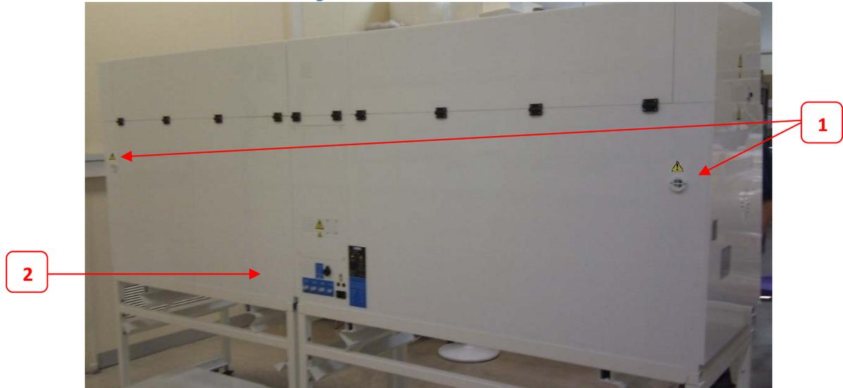
1. Secondary Pressure relief system vent
