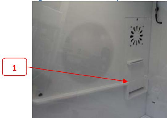
1. Water Tank Acces point for filling
