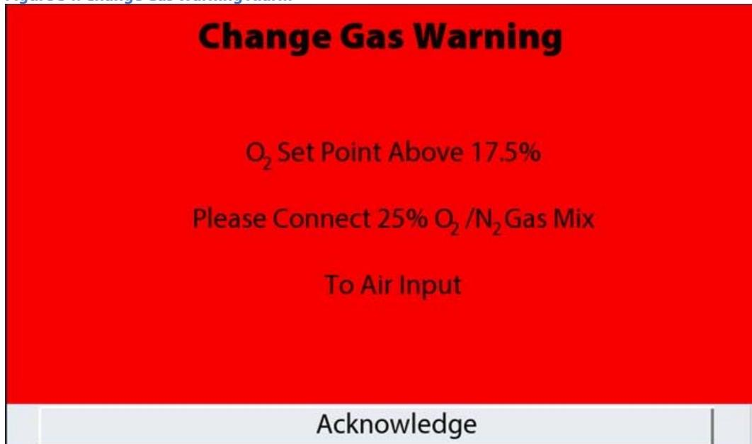
This alarm occurs when the O<sub>2</sub> set point has been set above 17.5% requiring the compressed air cylinder to be changed.
