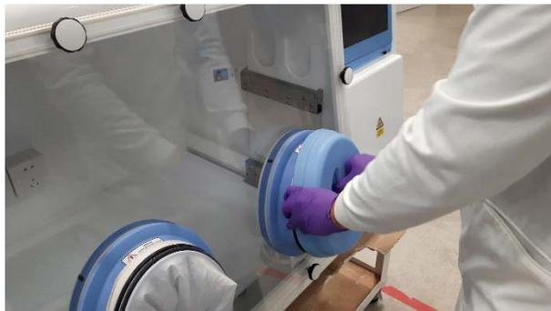
Note: Ensure that the cuffs are properly supported when exiting the workstation chamber. Failure to support the cuffs can cause the Ezee Sleeves to come off the glove ports. Note also that the Ezee Plugs must be correctly inserted into the cuffs, such that a gas tight seal is formed.
