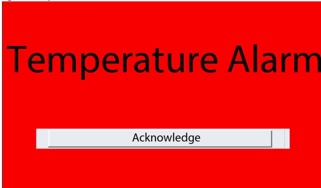
The alarm is turned off when the temperature returns to within +/- 1.0°C of the temperature setting.
