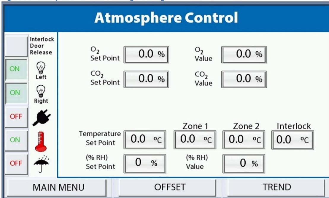
Each chamber is equipped with two internal lights (left and right). These are displayed by a light bulb on the Left Hand Side menu, one for the left light, and one for the right light.
