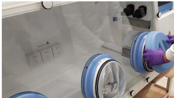
Note: Ensure that the cuffs are properly supported when exiting the workstation chamber. Failure to support the cuffs can cause the Ezee Sleeves to come off the glove ports.
