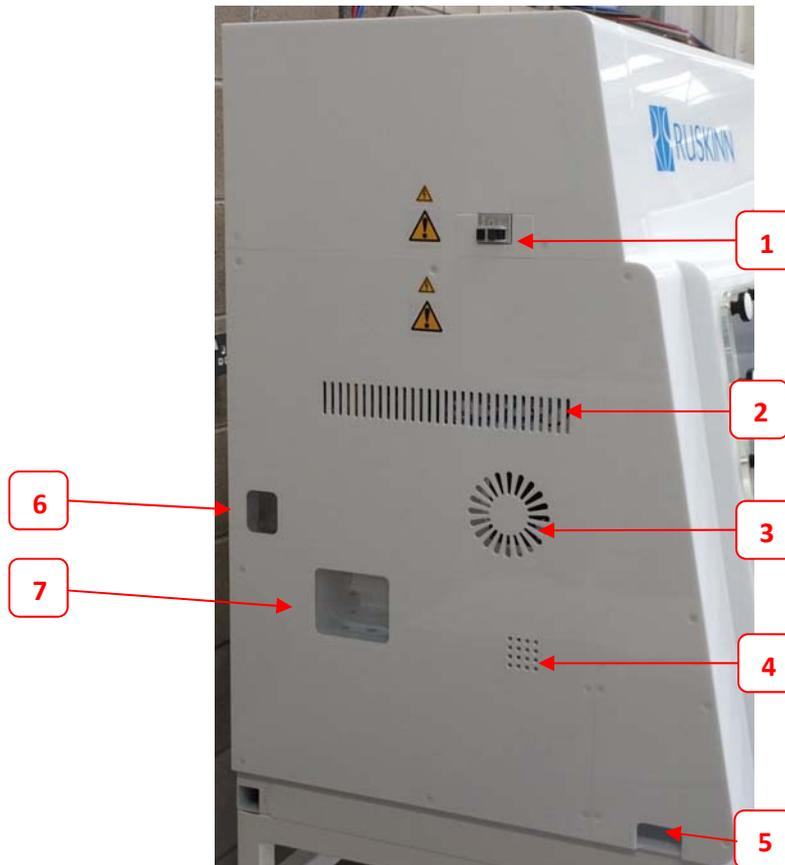
Figure 9: RCCB for the workstation
