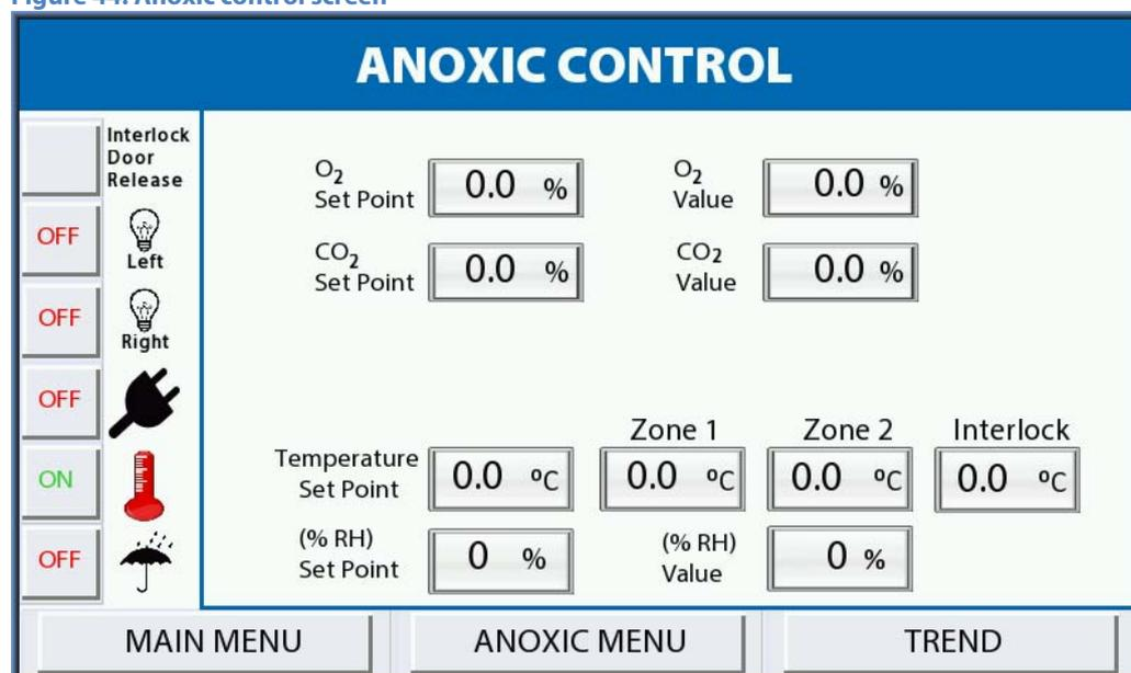
**O<sub>2</sub> Value:** This is the actual oxygen concentration in the workstation chamber.
