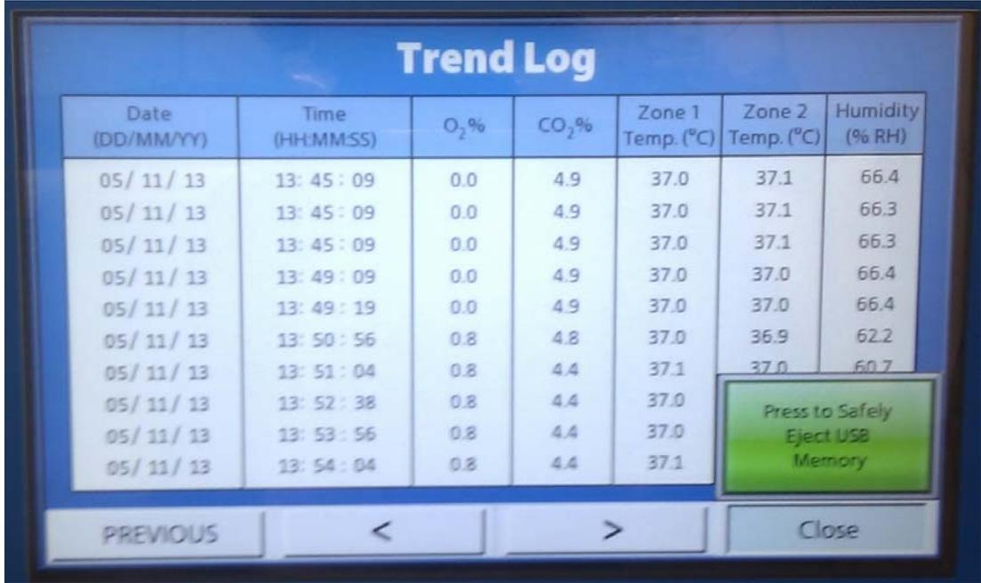
The Green **“Press to Safely Eject USB Memory”** button should be pressed to safely remove the USB stick. The Left USB stick contains the Left Hand Side Chamber Trend Log data, and the Right USB stick contains the Right Hand Side Chamber Trend Log data. Wait until the red **“USB has been ejected”** message to appear as shown in Figure 50, then remove the USB.
