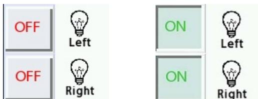
To switch off each light, touch the relevant left or right light bulb button, and the button will turn from displaying a green “ON” to red “OFF” and the internal light will be switched off.
