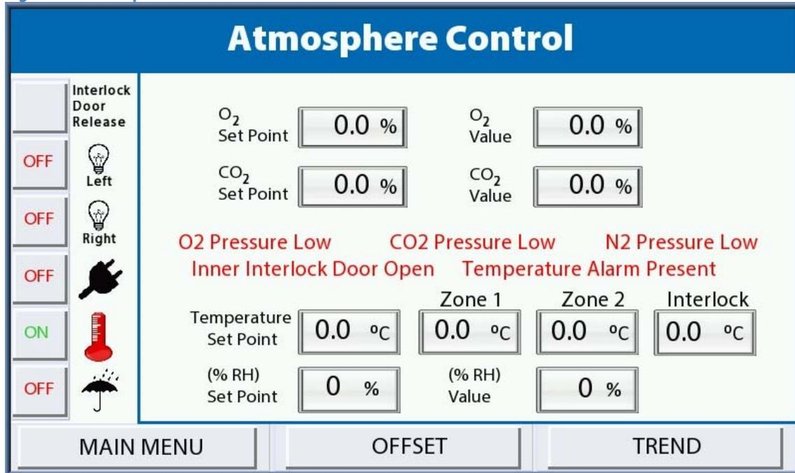
Figure 34: Change Gas Warning Alarm
