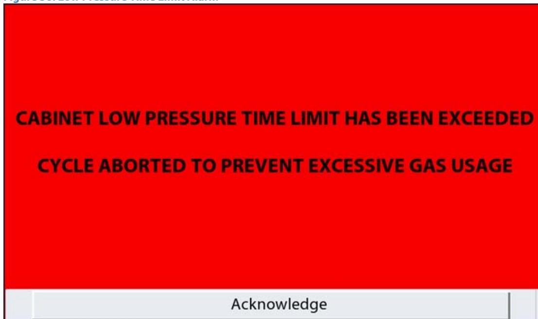
The low pressure time limit alarm occurs when the chamber has been unable to reach the required level over a set time period (15 minutes default). This could be due to glove ports being left off, leakage, or the incoming gas supply needing to be changed.
