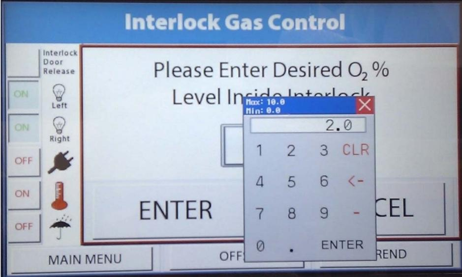
When the interlock door is closed a purge of the interlock will take place. The doors cannot be opened at this time and the following screens will be displayed.
