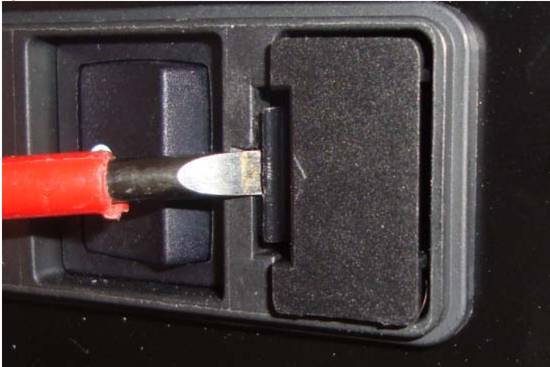
Figure 31: mains fuse holder removal
