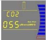
If Conductivity Units are chosen in CO1, then the Setpoint can be adjusted from 0.999  $\mu$ S/cm @25 °C to 0.055  $\mu$ S/cm @25 °C.
