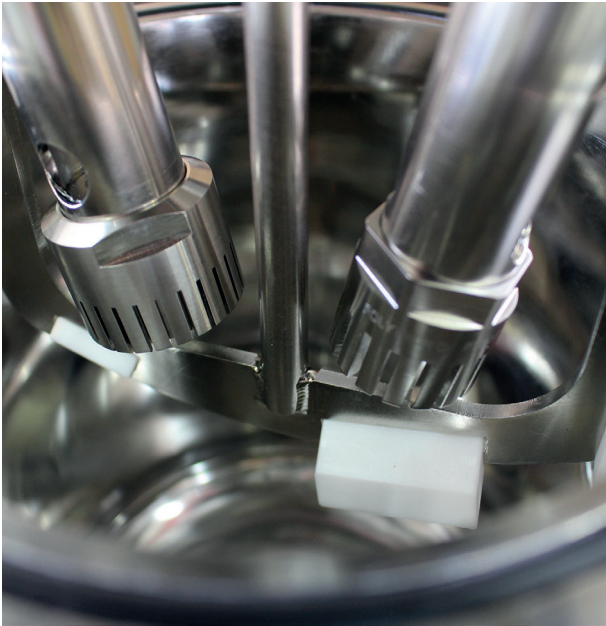
Design with two special dispersing aggregates
