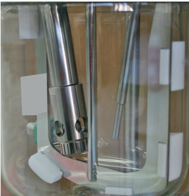
Dispersing aggregates, PTFE anchor stirrer and temperature probe
