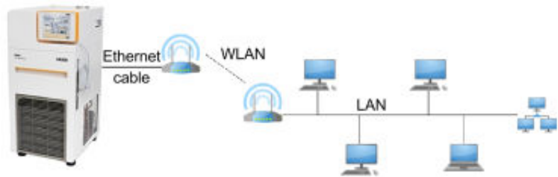
Fig. 16: Connected via LAN and WLAN
