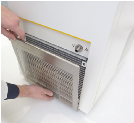
Fig. 72: Removing/attaching the front panel
