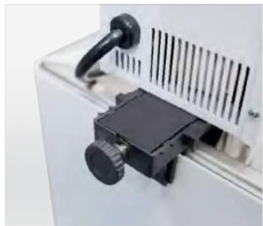
Screw clamp allows easy change to different bath vessels with a maximum wall thickness of 30 mm
