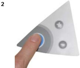
Press the Main Button once. The Display will show C02 and the Resistivity Setpoint value.
