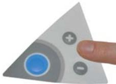
Press the "+" or "-" Button to match the volume Display to the volume measured.
