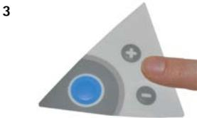
Press the "+" or "-" Button to adjust the Resistivity Setpoint from 1.0 MΩ.cm @25 °C to 18.0 MΩ.cm @25 °C.
