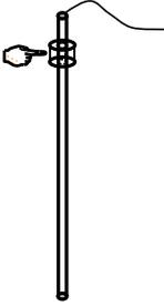
Move the Float on the Level Sensor to its highest possible position (representing a full Reservoir). Make sure the full water level is below the overflow port.
