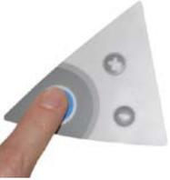
Press the Main Button 3 times. The Display will show C04. The highest Tank Level display will be blinking. This means that the highest water level is ready to be calibrated.
