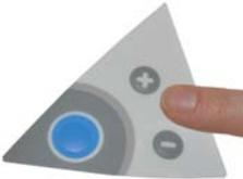
Press the "+" or "-" Button to adjust the exact amount of Product Water (in Litres) needed. Pre-set volumes of water can be adjusted from 0.25 L to 9.75 L in 0.25 increments.
