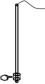
Move the Float on the Level Sensor to its **lowest** position (representing an empty Reservoir). Press LOW.
