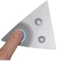
Press the Main Button 4 times. The Display will show C05 and "0" days left on the UV Timer.
