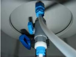
Connect the 6mm diameter tubing via an 8 to 6mm fitting to the bottom of the Reservoir and the level sensor of the tank to the level sensor jack input
