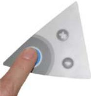
Press the Main Button 4 times. The Display will show C05 and the days left on the UV Timer.
