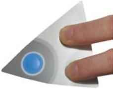
Press the "+" and "-" Buttons together to enter the highest water level. The Signal Voltage at that position becomes defined as the '100%' position. The Display will show the lowest Tank Level (red level) display blinking.
