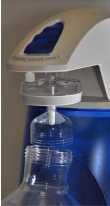
How to Calibrate the Flowrate from the Direct-Q System (F02) Measure the total volume of water (in Litres) dispensed from the system using a 1 L graduated cylinder.
