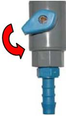
Open the Tank Outlet Valve. Allow the tank to be emptied to its lowest water level.
