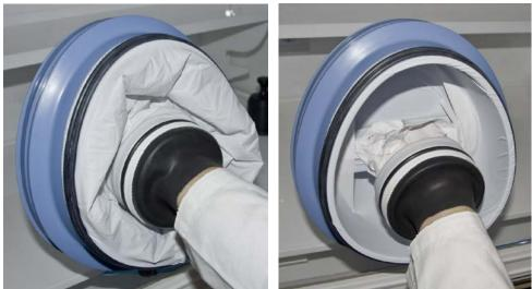
Figure 22: Sleeve before and after vacuum operation
