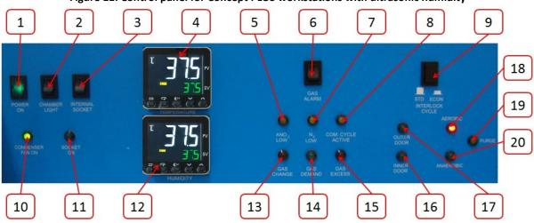
Figure 11: Control panel for Concept PLUS workstations with ultrasonic humidity
