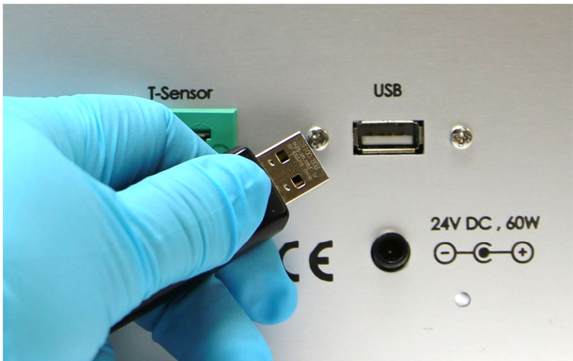
How to plug in USB drive:
