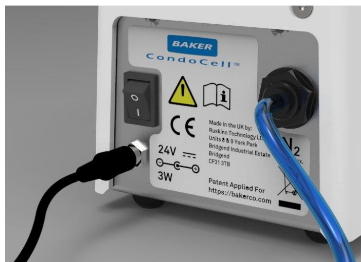
Figure 26 - Purge Unit Power Connection
