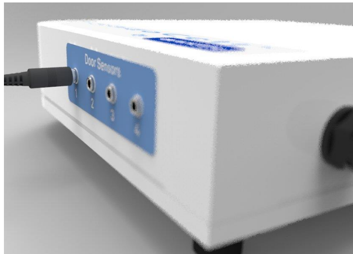
Figure 15 - ACU Sensor Cable Connection
