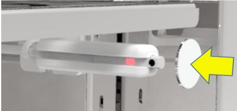
Figure 29 - Checking Sensor Alignment & Operation
