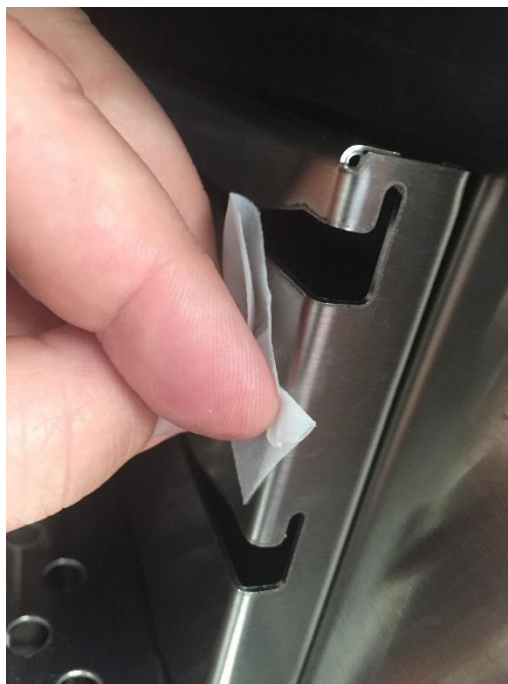
Figure 17 - Cleaning Surface for Sensor Adhesion
