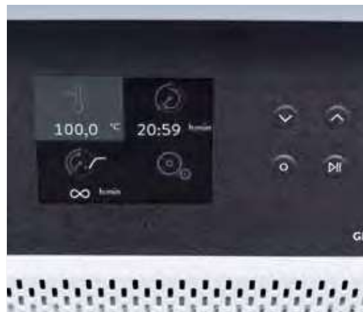
Large, high-contrast TFT display with menu-guided controls
