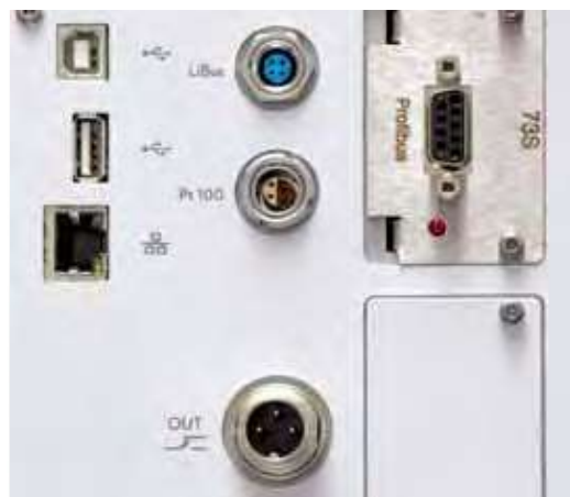
Ethernet, USB, malfunction contact and Pt100 as standard, two module slots for additional interfaces
