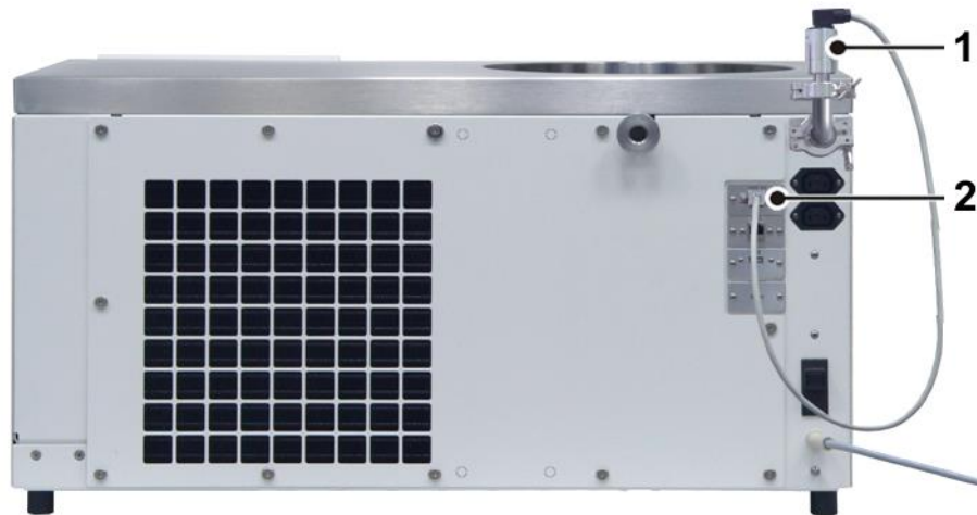
Fig. 14: Position of the vacuum sensor and the connection socket
