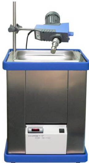
Fig. 10: Cooling bath with spin freezing device
