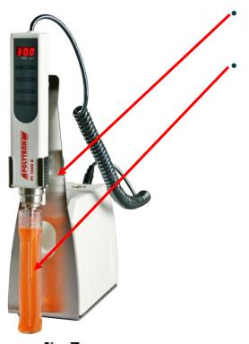
Plate stand ST-P15/320 with base station and handheld unit holder (accessory)
