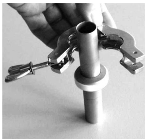
Fig. 79: Attaching the clamping ring
