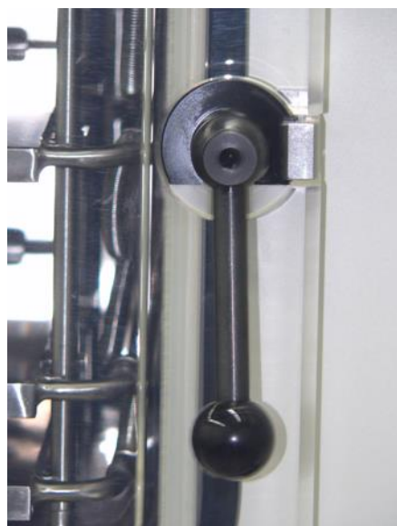
Fig. 23: Example of a door locking system of the loading door; here: door stop (left side)
