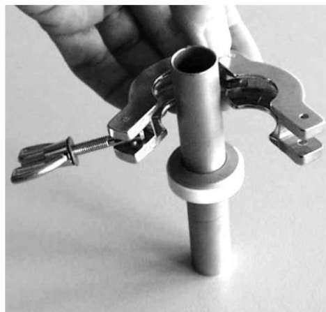
Fig. 78: Attaching the clamping ring
