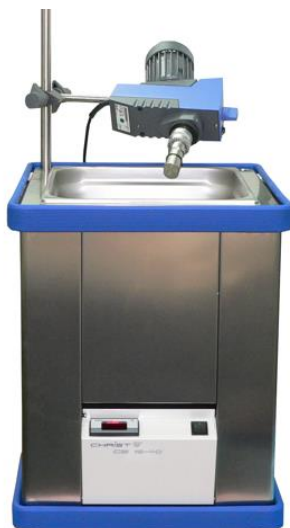
Fig. 13: Cooling bath with spin freezing device
