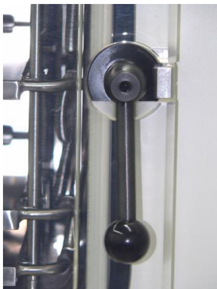
Fig. 21: Example of a door locking system of the loading door; here: door stop (left side)
