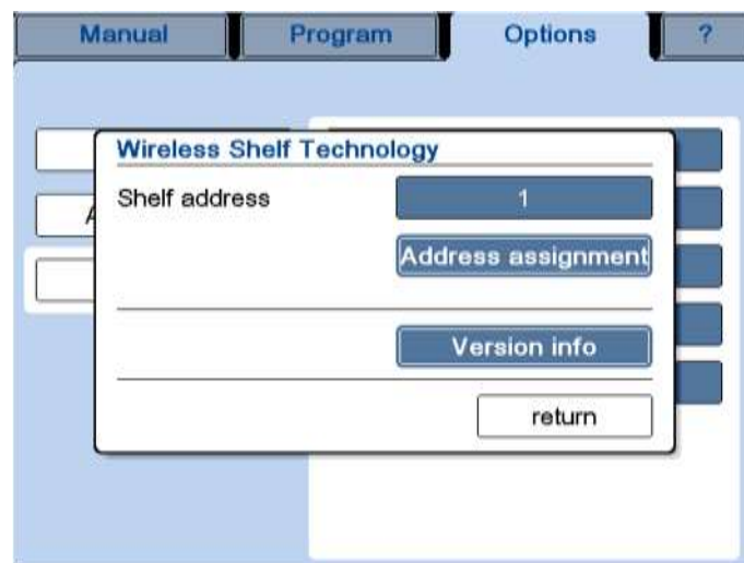
Fig. 49: Wireless shelf technology – assignment of shelf addresses
