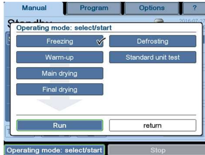
Fig. 32: Dialog box "Operating mode: select/start" (The version of the dialog box that is displayed depends on the equipment of the freeze-dryer.)
