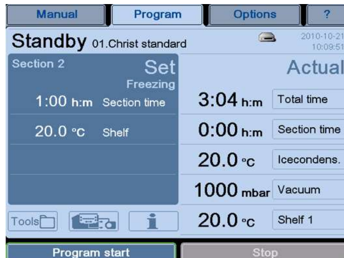
Fig. 69: The freeze-drying process can be started with the aid of the button "Program start".
