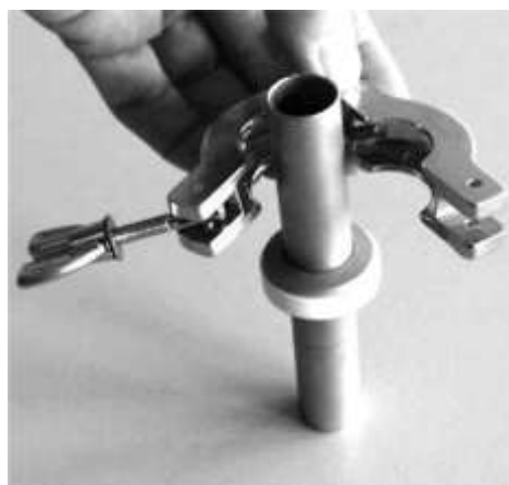
Fig. 72: Attaching the clamping ring
