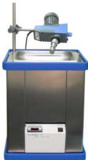
Fig. 11: Cooling bath with spin freezing device
