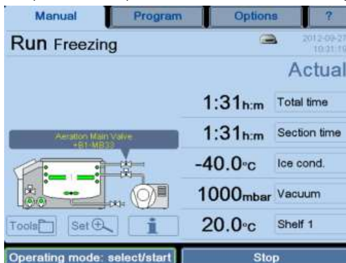
Fig. 28: Schematic system diagram with the name and reference designator of the component
