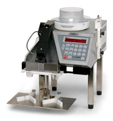
The KL50ic/icf are ideal for facilities that need absolute accuracy when batch-counting tablets and identical-shaped items
