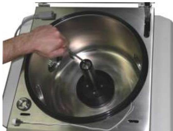
Fig. 58: Loosening the rotor shaft incl. magnetic coupling
