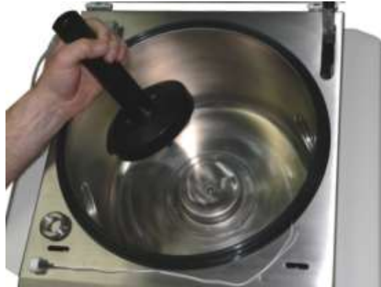
Fig. 59: Removing the rotor shaft incl. magnet coupling
