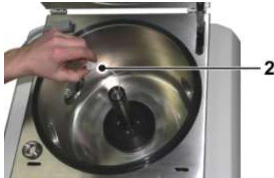
Fig. 57: Removing the electronic temperature measurement system
