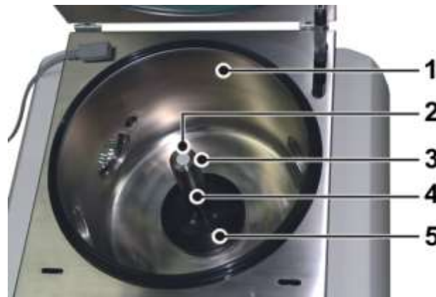
Fig. 53: Rotor chamber with rotor shaft incl. magnet coupling
