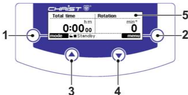
Fig. 18: User interface of the CDplus control system
