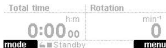
Fig. 19: Display of the assignment of the function keys; here: left key "mode", right key "menu"
