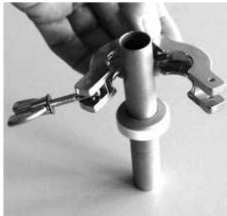
Fig. 51: Attaching the clamping ring
