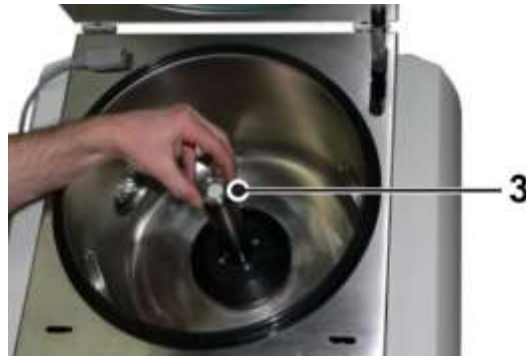
Fig. 56: Removing the cap
