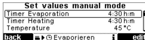
Fig. 29: Manual mode – selecting a set value
