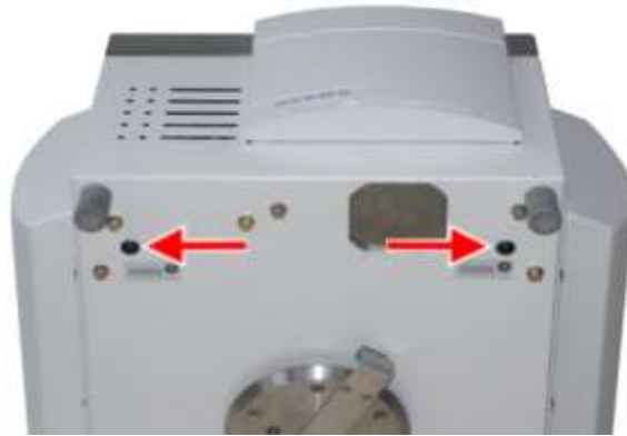
Fig. 46: Position of the plastic screws of the emergency lid release
