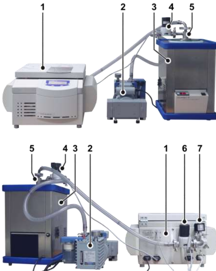
Fig. 11: Combination of the RVC with vacuum pump and cooling trap (front view)
