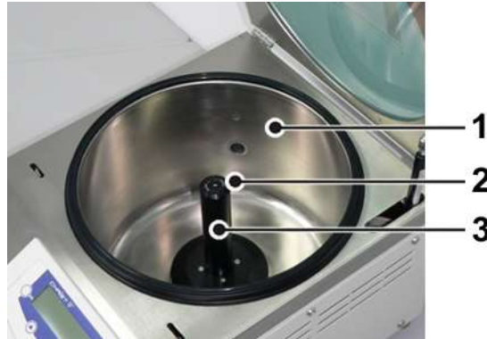
Fig. 54: Rotor chamber with rotor shaft
