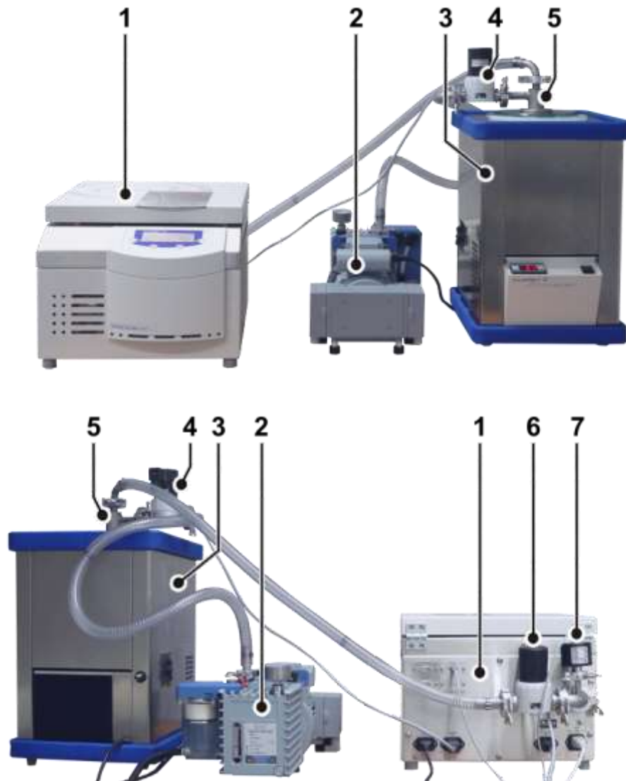
Fig. 12: Combination of the RVC with vacuum pump and cooling trap
