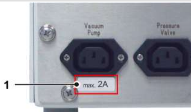
Fig. 10: Indication of the maximum current for the vacuum pump (example)
