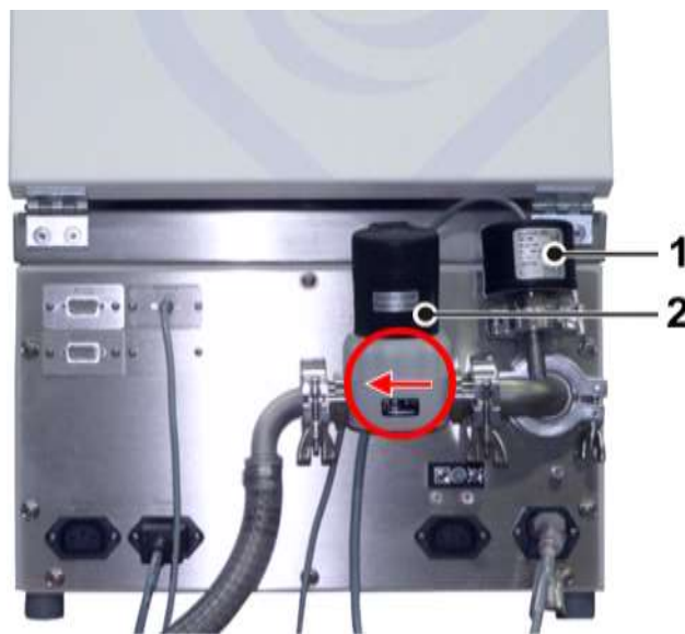
Fig. 9: Installation of the pressure control valve and the vacuum sensor
