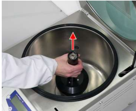
Abb. 56: Removing the rotor shaft
