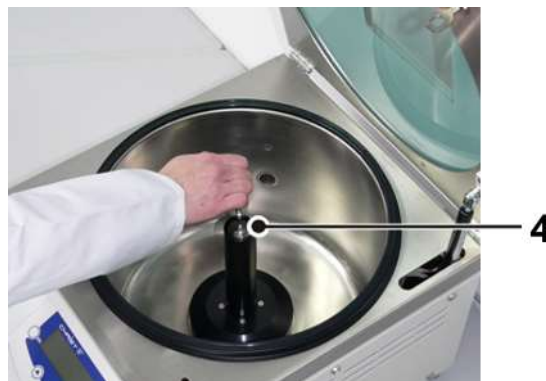
Fig. 55: Removing the countersunk screw
