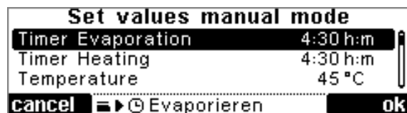
Fig. 31: The selected set value is displayed in an inverted manner
