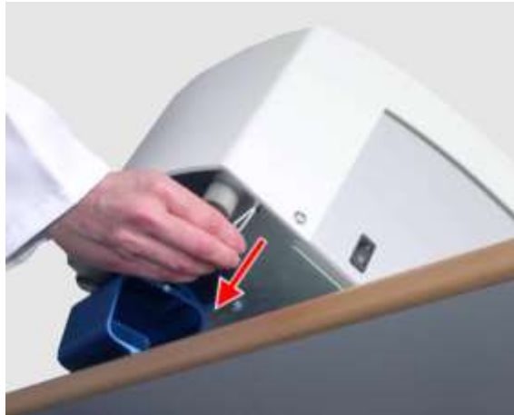
Fig. 38: Unlocking the lid locks
