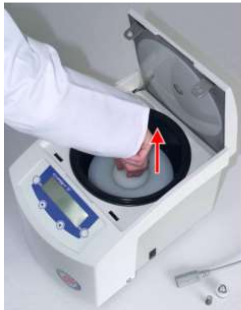
Fig. 46: Removing the rotor shaft
