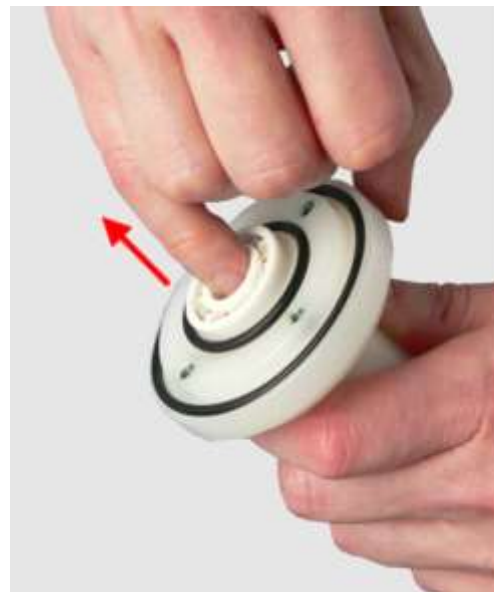
Fig. 50: Removal of the lower ball bearing
