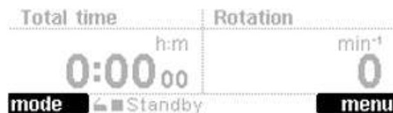
Fig. 18: Display of the assignment of the function keys; here: left key "mode", right key "menu"
