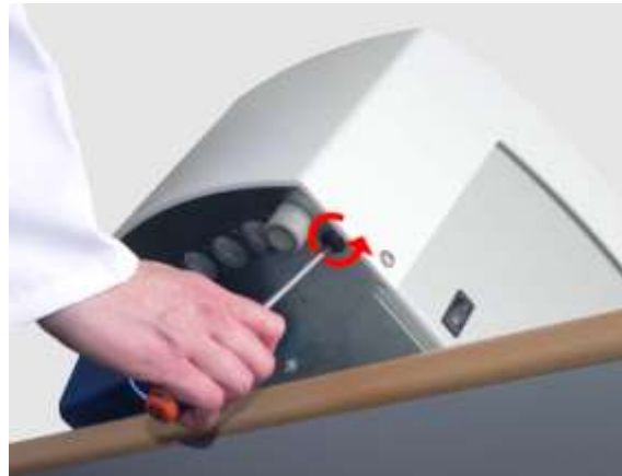
Fig. 36: Loosening of the plastic screw
