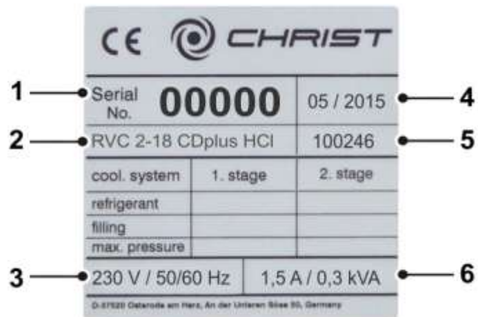
Fig. 2: Example of a name plate
