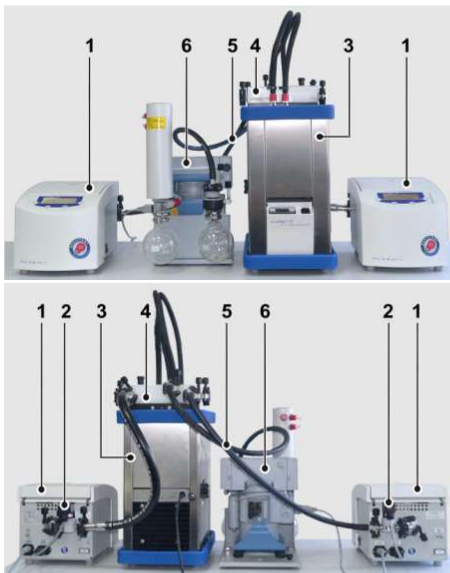
Fig. 4: Combination of two RVCs with a vacuum pump and cooling trap with a distributor block, front and rear view
