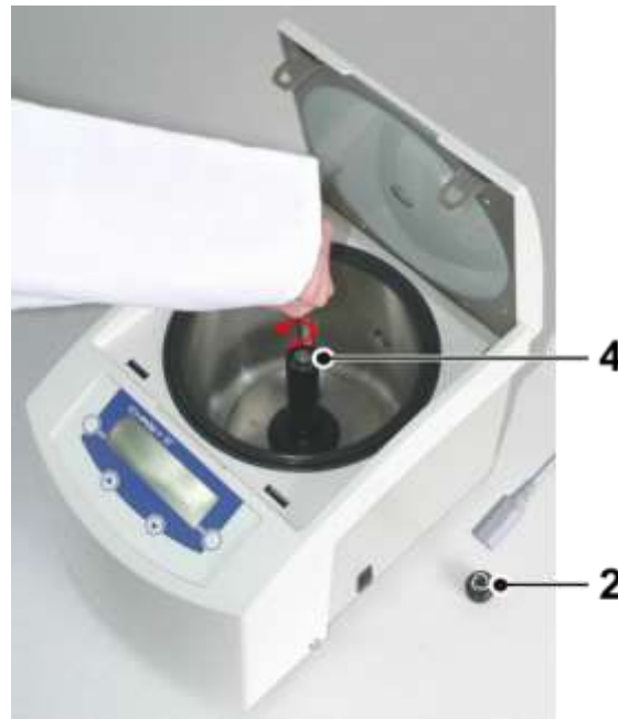
Fig. 43: Removing the countersunk screw
