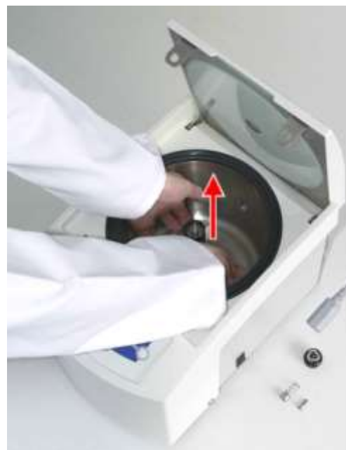
Fig. 44: Removing the rotor shaft
