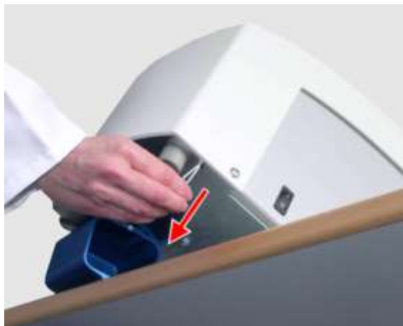
Fig. 37: Unlocking the lid locks
