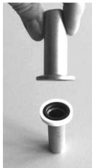
Fig. 39: Small flange with centring ring and small flange
