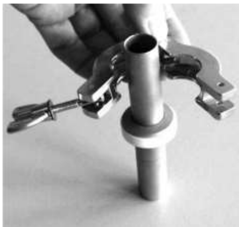
Fig. 40: Attaching the clamping ring
