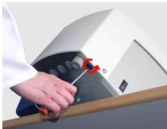
Fig. 35: Loosening of the plastic screw
