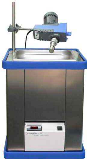
Fig. 11: Cooling bath with spin freezing device
