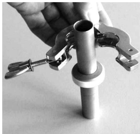
Fig. 71: Attaching the clamping ring
