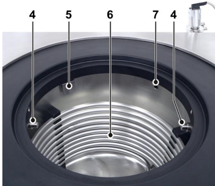
Fig. 3: Ice condenser chamber
