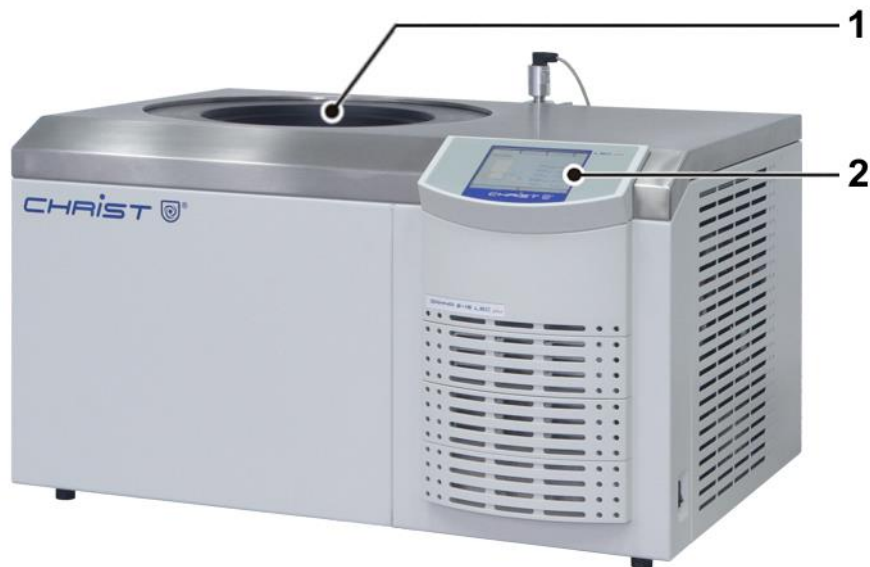
Fig. 1: Total view of the freeze-dryer
