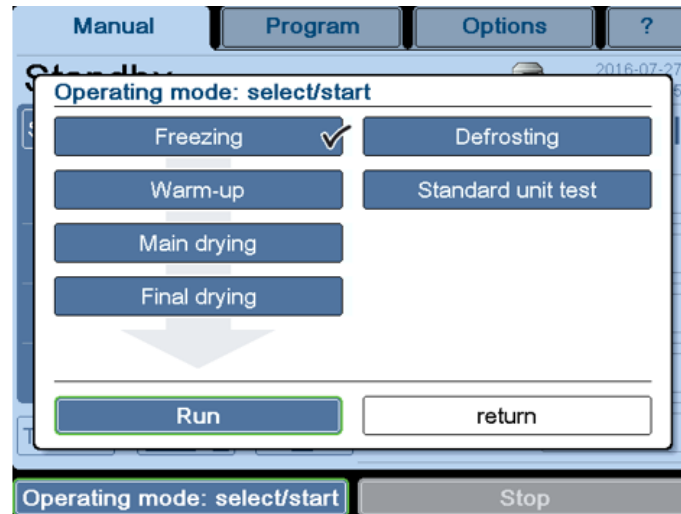
Fig. 31: Dialog box "Operating mode: select/start" (The version of the dialog box that is displayed depends on the equipment of the freeze-dryer.)
