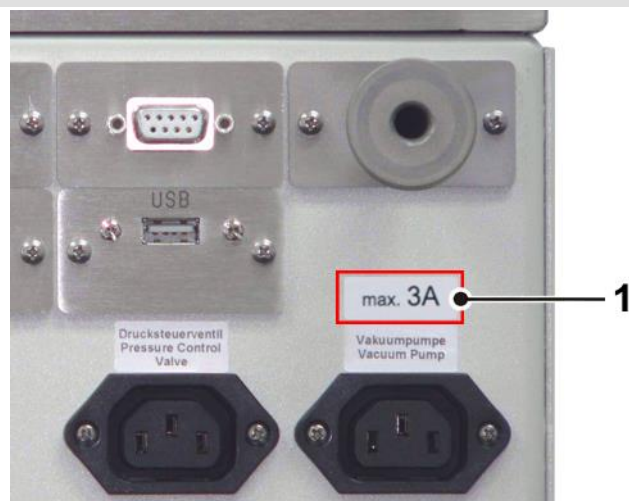
Fig. 16: Indication of the maximum current for the vacuum pump (example)
