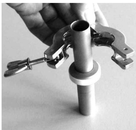
Fig. 71: Attaching the clamping ring
