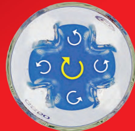
GS vessel principle (viewed from above)
