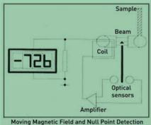
Both MK1 and the AUTO work on the basis of stationary sample and moving magnets. Two pairs of magnets are placed at opposite ends of a beam making a balanced system having a magnetic field at each end. Introduction of the sample into the magnetic field attempts to deflect the beam and the
