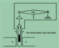
The traditional technique, developed by employs a conventional balance and a large permanent magnet. The magnet remains stationary while the sample is caused to move, giving apparent gain or loss in sample weight
