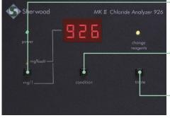
1926 Factor Button Factor conversion to Salt concentration. (926S Switch Selects sample volume 100µl/20µl).
