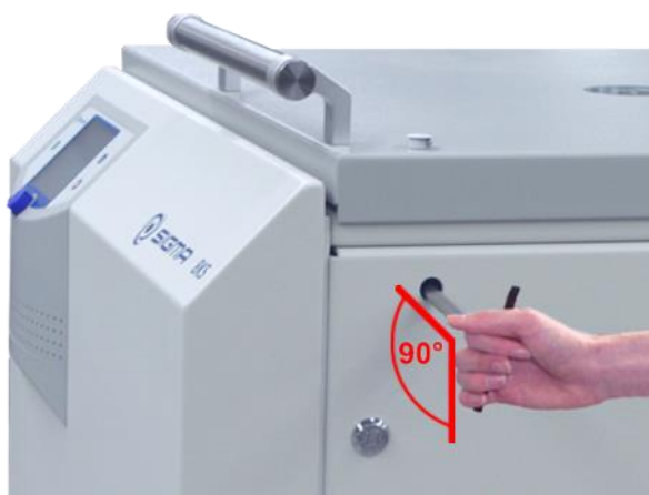
Fig. 44: The emergency lid release key must be inserted horizontally.
