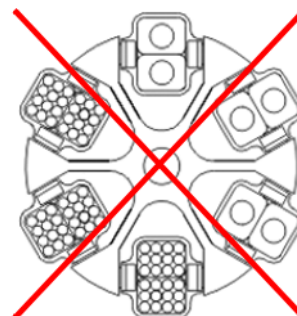
Fig. 19: Permissible and impermissible loading of a swing-out rotor with vessels of various sizes (example illustration)
