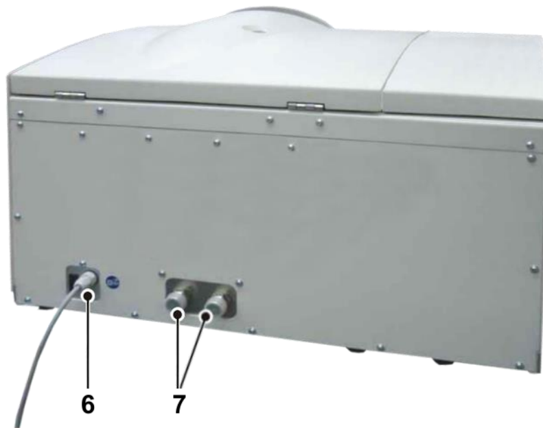
Fig. 3: Rear view of a water-cooled centrifuge (GMP version)
