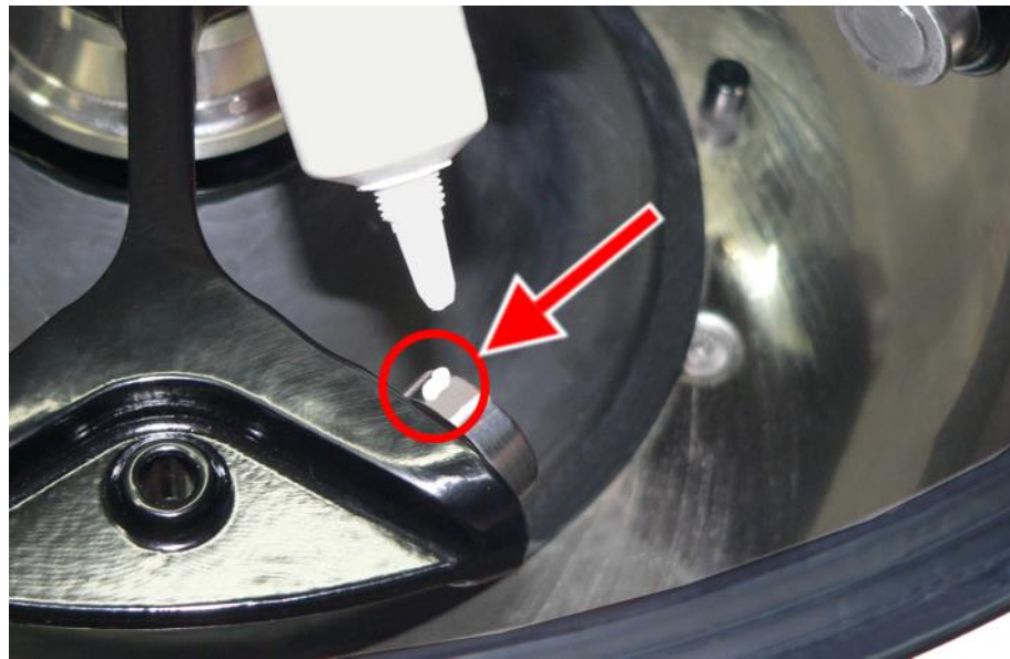
Fig. 35: Sufficient quantity of grease for one bolt
