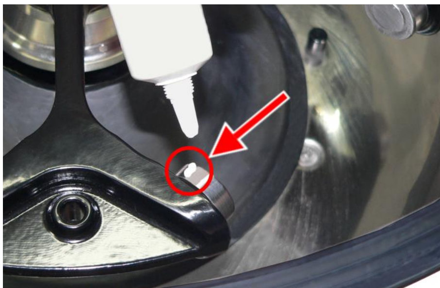
Fig. 32: Sufficient quantity of grease for one bolt
