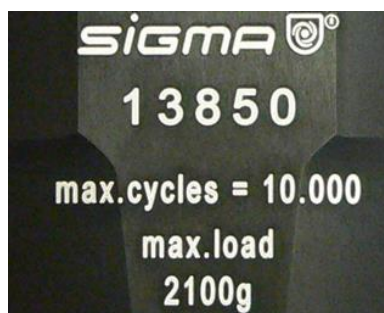
Fig. 4: Different service life – engraving on the bucket/rotor
