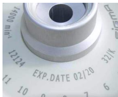
Fig. 4: Different service life – engraving on the bucket/rotor
