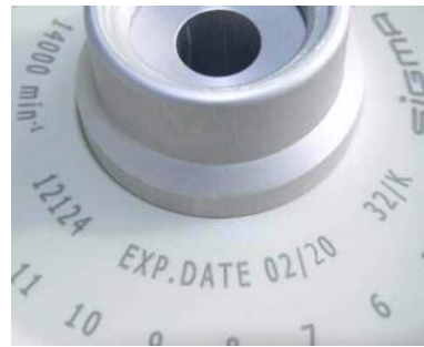
Fig. 4: Different service life – engraving on the bucket/rotor
