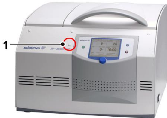
Fig. 29: Position of the opening for the emergency lid release
