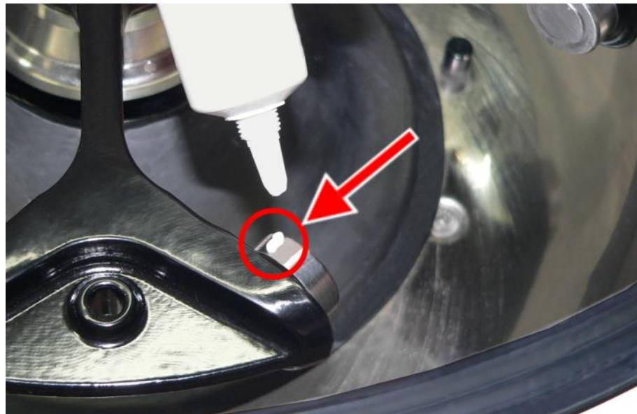
Fig. 29: Sufficient quantity of grease for one bolt
