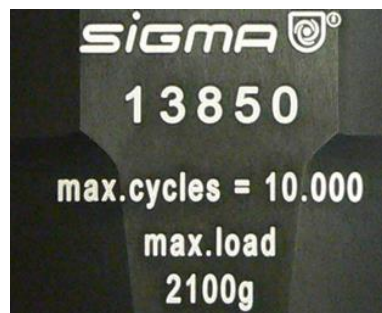
Fig. 4: Different service life – engraving on the bucket/rotor
