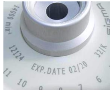
Fig. 4: Different service life – engraving on the bucket/rotor
